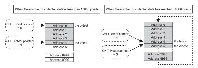
The head pointer does not change until CHI Logging data (Un\G5000 to Un\G44999) becomes full after the logging start (The value is fixed to 0). The head pointer moves by one point when CHI Logging data (Un\G5000 to Un\G44999) becomes full and the overwriting of data starts from the first address.
