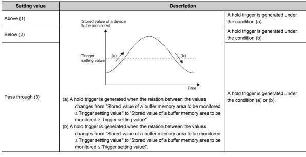
Set a value where a hold trigger is generated to CH□ Trigger setting value (Un\G1082 to Un\G1085).
