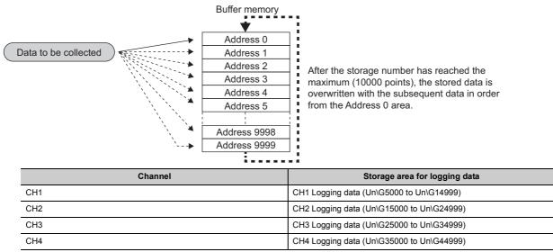
If logging has been performed even once, all data in CHI Logging data (Un\G5000 to Un\G44999) are cleared to 0 when Operating condition setting request (Y9) is turned off and on.
