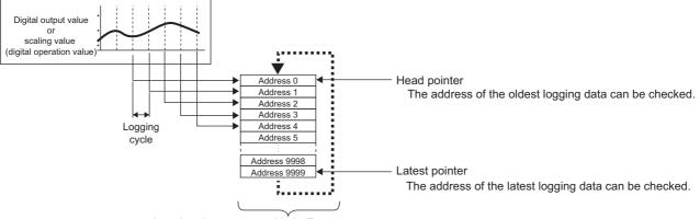
Logging data are stored in buffer memory areas. After the storage number has reached the maximum (10000 points), the stored data is overwritten with the subsequent data in order from the Address 0 area.
