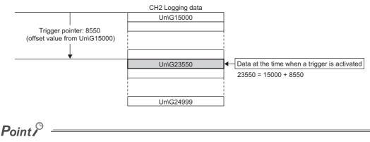
When CHI Logging hold request (Un\G1008 to Un\G1011) is changed from On (1) to Off (0), CHI Trigger pointer (Un\G1114 to Un\G1117) is cleared to zero.
