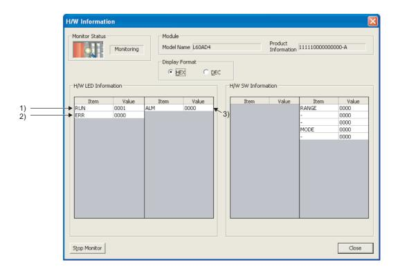
11.7 Checking the Status of the A/D Converter Module by the System Monitor
