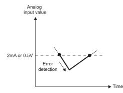
The setting for CHD Input signal error detection setting value (Un\G142 to Un\G149) is ignored.
