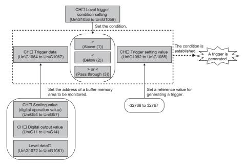
For example, to generate a hold trigger when a value in CH1 Digital output value becomes greater than 10000, configure settings as follows.
