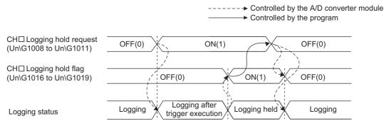
Logging does not stop when Off (0) is set to CH□ Logging hold request (Un\G1008 to Un\G1011) before On (1) is stored in CH□ Logging hold flag (Un\G1016 to Un\G1019).
