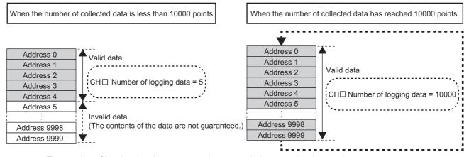
The number of logging data increases one by one each time new data is stored. When  $CH\square$  Logging data (Un\G5000 to Un\G44999) becomes full (Number of logging data = 10000), the next data is stored in the first address of  $CH\square$  Logging data (Un\G5000 to Un\G44999), and the logging operation continues overwriting the existing data. The number of logging data is fixed to 10000.
